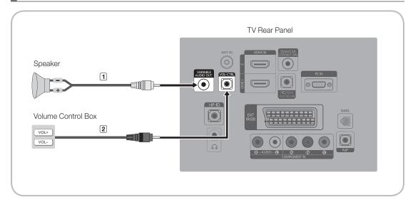
1. Connect the VARIABLE AUDIO OUT port of the TV to the Bathroom Wall Speakers of the hotel.
